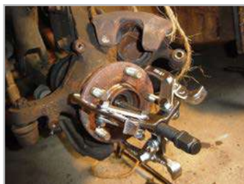
3 Jaw Puller used for removing tyre hub
