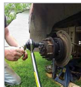
Torque multiplier used for lug nuts
