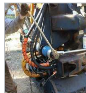
Torque multiplier used for machine nut tightening
