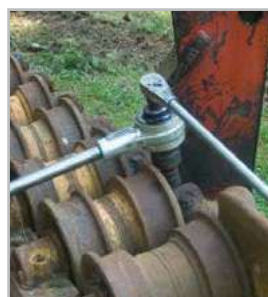
Torque multiplier used on tracks
