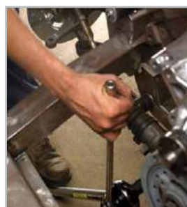
Torque multiplier used in inaccessible areas
