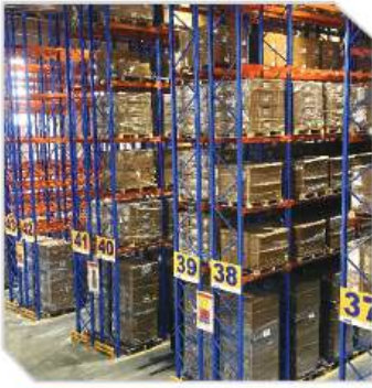
Selective Pallet Racking
