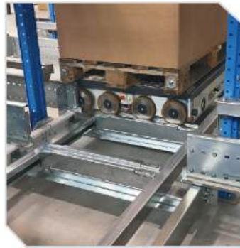
4 Way Pallet Shuttle ASRS
