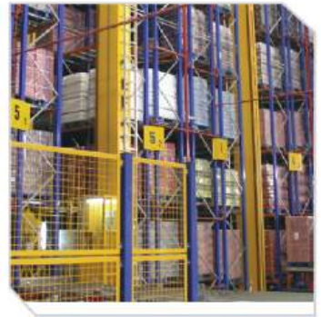
AS/RS with Stacker Crane
